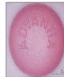
Surface Roughness Value: Sq = 5.41 A. Tablet Coated with Advantia® Preferred HG Coating
